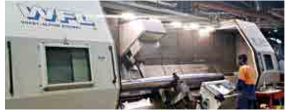
PICTURED ABOVE: Hofmann's latest M100 5-axis multifunctional CNC lathe machining a complete apron feeder drive shaft.
