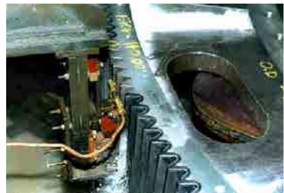
Computerised full contour induction hardening of large Slew gears and bearing race ways.
