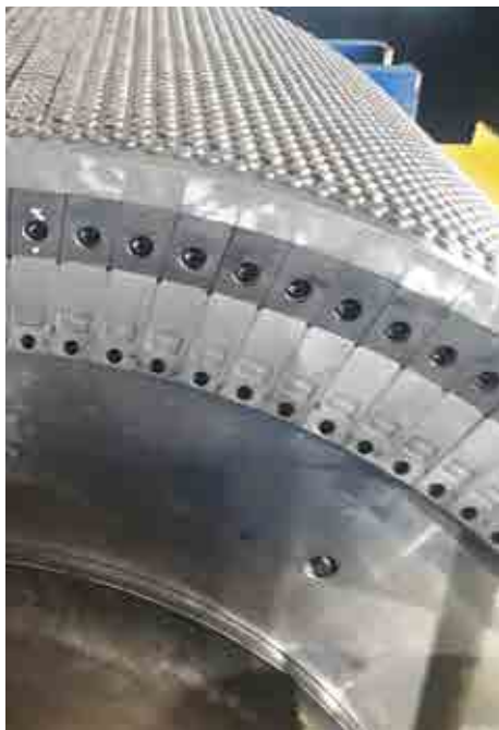
Tungsten carbide blocks, bolt on retaining clamp plates and soldered Tungsten Carbide pieces (Patent no: 2011301142). • Individually clamped • Can't break off • Individual blocks can be replaced.
