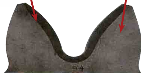
Section tested piece showing the induction hardened profile.
