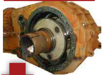
Old bucket wheel gearbox
