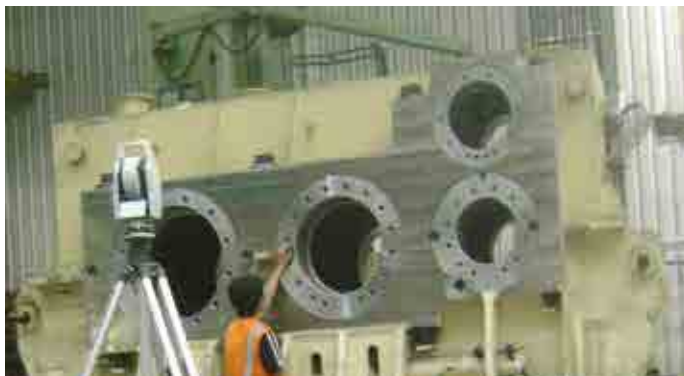
LASER TRACKER ON A GEARBOX CASING
