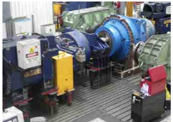
Above: Hofmann refurbished P2SA-38 (2800kW) HPGR Gearbox under load test.
