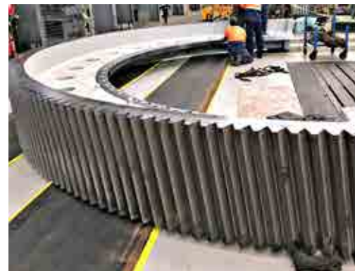
PREPARING FOR FINAL MACHINING
